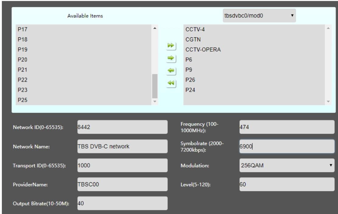
Frequency: this DVBC modulator card is a little special in frequency setting. For a same card, once the 1<sup>st</sup> RF device frequency is setting the rest 3 RF device will be set. This depends on Modulate chipset characteristic. For example, “tbsdvbc0” set to “474Mhz”; the 2<sup>nd</sup> “tbsdvbc1” will be “482Mhz”; the 3<sup>rd</sup> “490Mhz”; and the 4<sup>th</sup> “498Mhz”. Step is 8Mhz.
